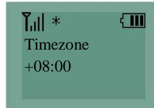
*According to the **GMT** got from satellite and the **timezone** you set, ManGo displays **correct** date and time on Date/Time interface.*
